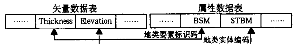
图 4 矢量数据表与属性数据表的链接 Fig.4 Link between table of vector data and table of attribute data
